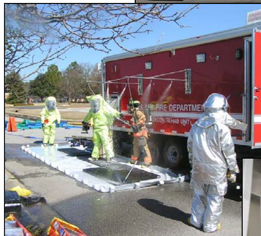
Above: DoD Fire Academy (Goodfellow) Mass Casualty Decontamination trailer. Left: Exterior decon station with stainless steel booms for non-ambulatory or technical decon. Below: Interior decon station with stainless steel, multi-nozzle, full body shower.
