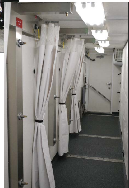
Above: DoD Fire Academy (Goodfellow) Mass Casualty Decontamination trailer. Left: Exterior decon station with stainless steel booms for non-ambulatory or technical decon. Below: Interior decon station with stainless steel, multi-nozzle, full body shower.
